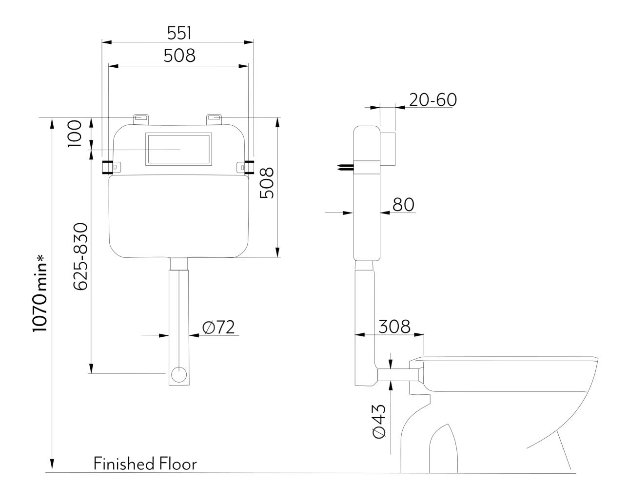
\*Cutting the flush pipe (#6-See parts list) below minimum recommended dimension, may result in reduced flush force.
